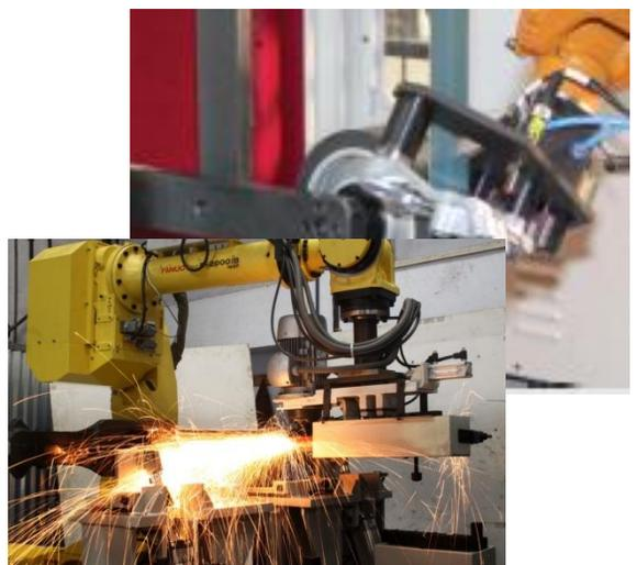
Disruptive Technology - Robotic Deflashing and Fettling for Foundry
